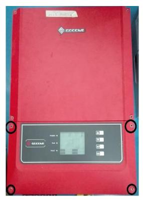
3) Remove the 4 screws on the screen and take off the screen.
